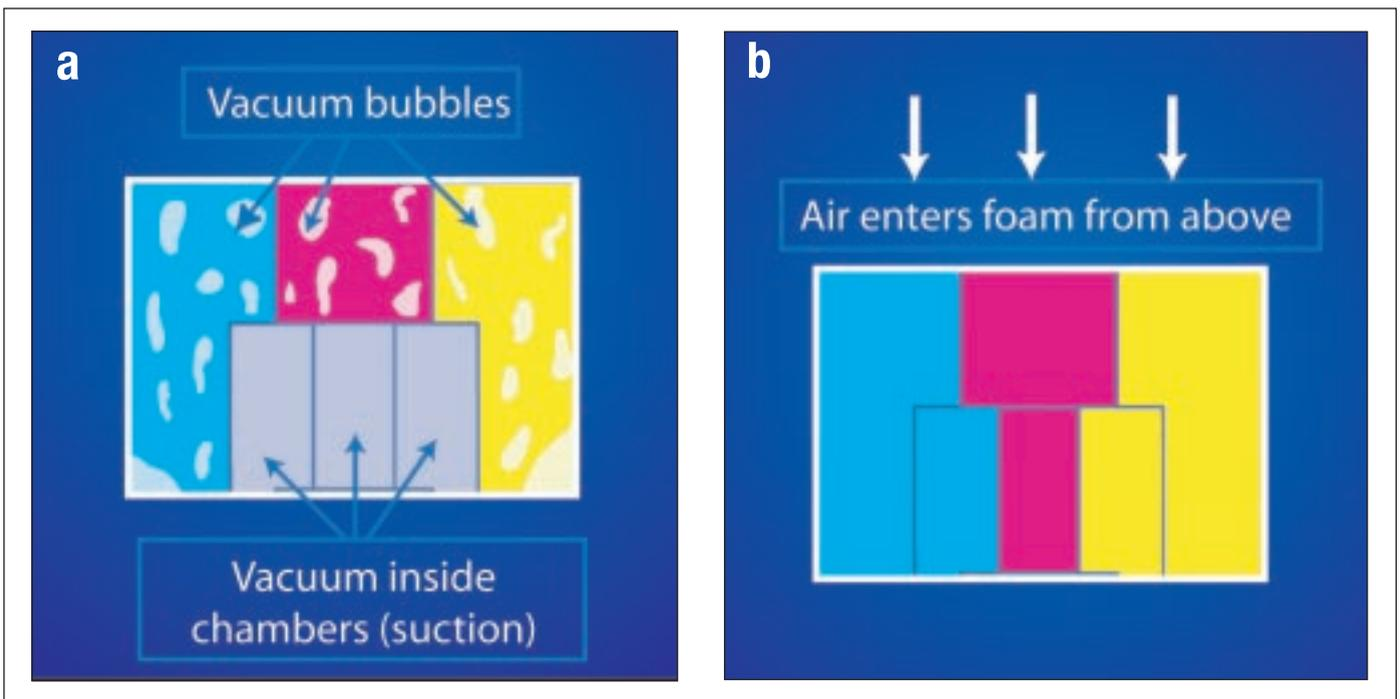
Figures 8a and 8b. Schematic illustration showing the filling process under vacuum. Figure 8a. After cartridge filling under vacuum, the foams contain ink and some small vacuum bubbles, and the chambers that lead the ink to the print head are also under vacuum. Figure 8b. When air is released into the filled cartridge from above, all vacuum areas suck ink inside, and the foams and chambers will be free of air.
