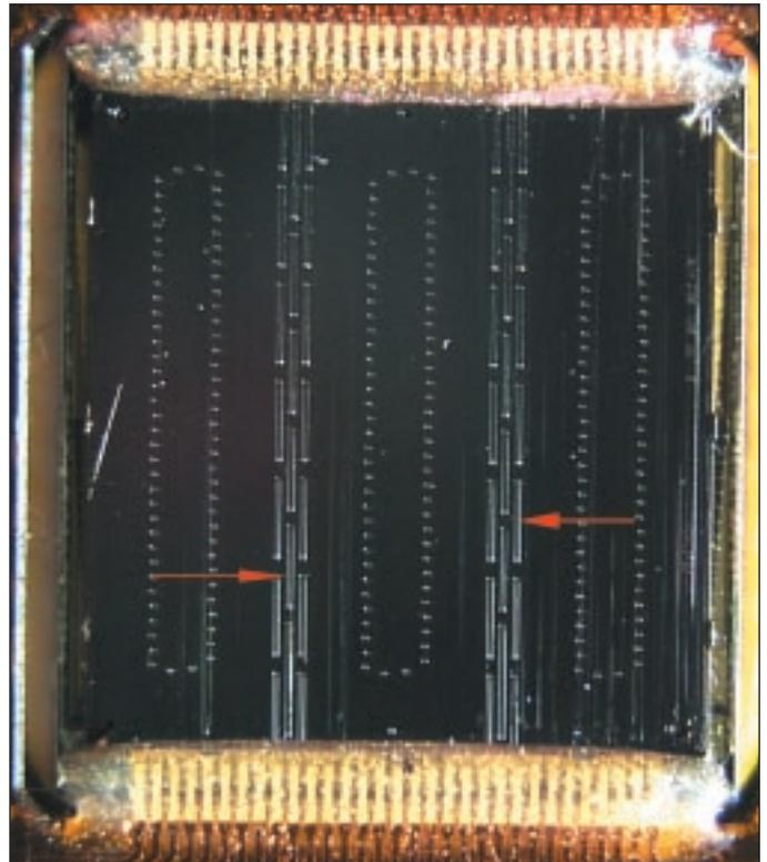
**Figure 1. Macro-image of a HP 641 nozzle plate, which is made from palladium and nickel. The nozzle plate has 68 nozzle holes for each color. Additionally, there are two rows of vertical cuts in the nozzle plate (see red arrows).**
