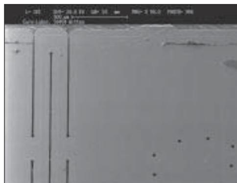
**Figure 2.** SEM image of a 641 nozzle plate. Some nozzles and one row of three parallel cuts at higher magnification.
