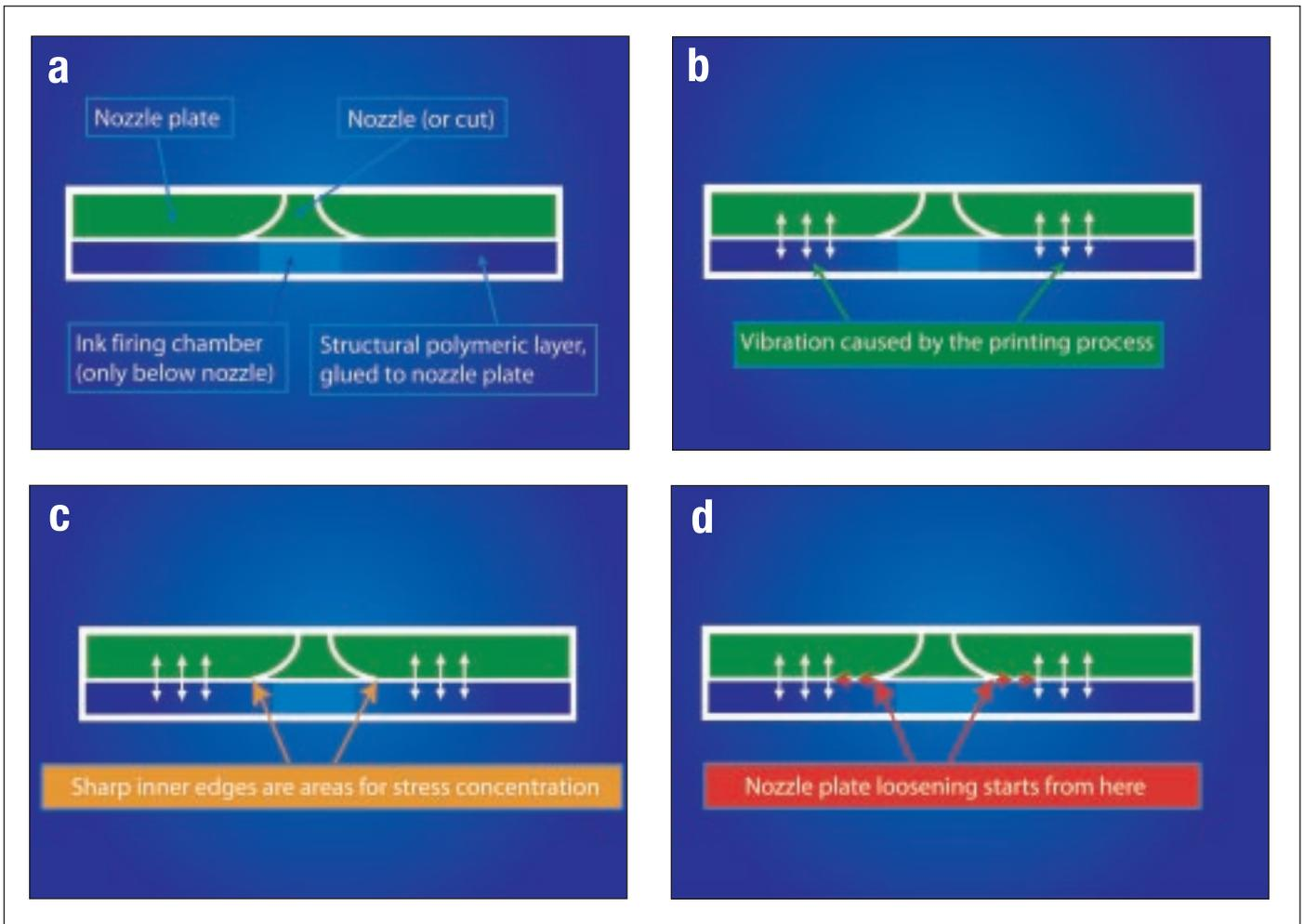
**Figure 4. Schematic illustration of the nozzle plate loosening process in four steps (a-d) caused by print-head vibration during the printing process. The result is slow and continuous loosening of the nozzle plate, which initiates around the nozzles and cuts and grows until it reaches the outside of the nozzle plate. Also see the images in Figure 5.**
