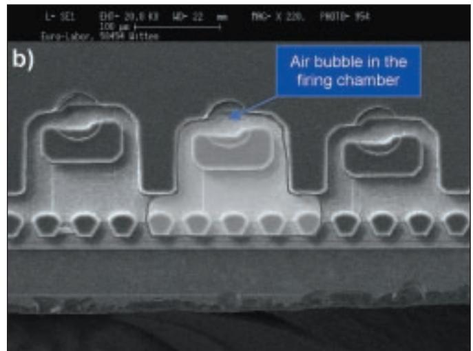
**Figure 7. SEM image of three ink firing chambers in a HP 6578 print head. An additional schematic illustration shows how the air bubble coming from the air chambers (shown in Figure 6) enters the print head (a) and causes interruption of the ink flow after entering the firing chambers (b).**
