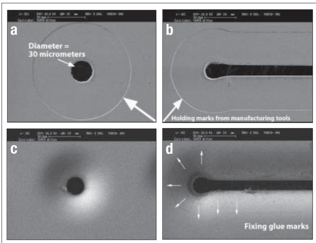
**Figure 3.** SEM images of a 614 nozzle plate presenting a nozzle and a cut. Figures 3a and 3b. View from the outside of the cartridge with sharp edges at nozzle and cut, and showing holding marks from a manufacturing tool. Figures 3c and 3d. View from inside (towards the print head) showing clearly that the inner edges are rounded. Note that the magnification of Figure 3a is higher, which is what makes the nozzle hole seem to be larger than in the other images.
