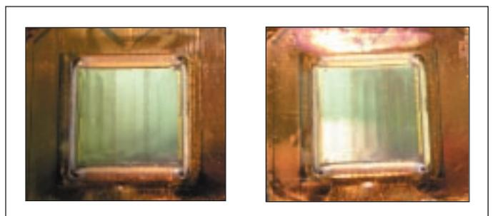
**Figure 5. The beginning of nozzle plate loosening can be detected by observation of surface undulations around the nozzle groups and cuts.**
