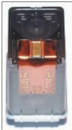
**Figure 1. Overview of the 629 cartridge print head.**
