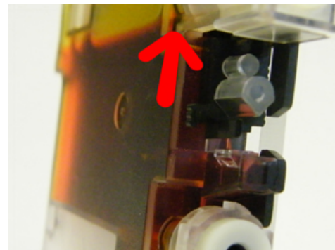
Push reflector up as shown before installing cartridge into printer.
